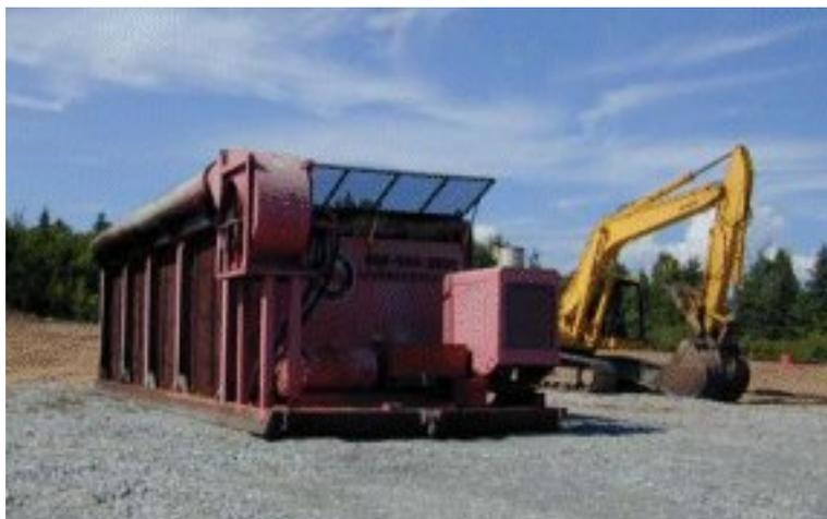
**The high efficiency air burner unit used to incinerate infested trees**
